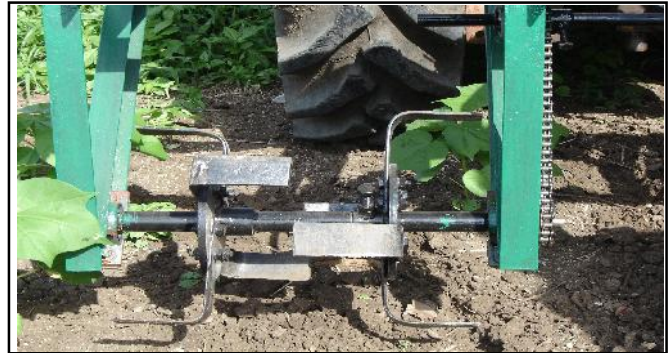
Fig. 1 : Operation of inter-row rotary weeder in row crop
