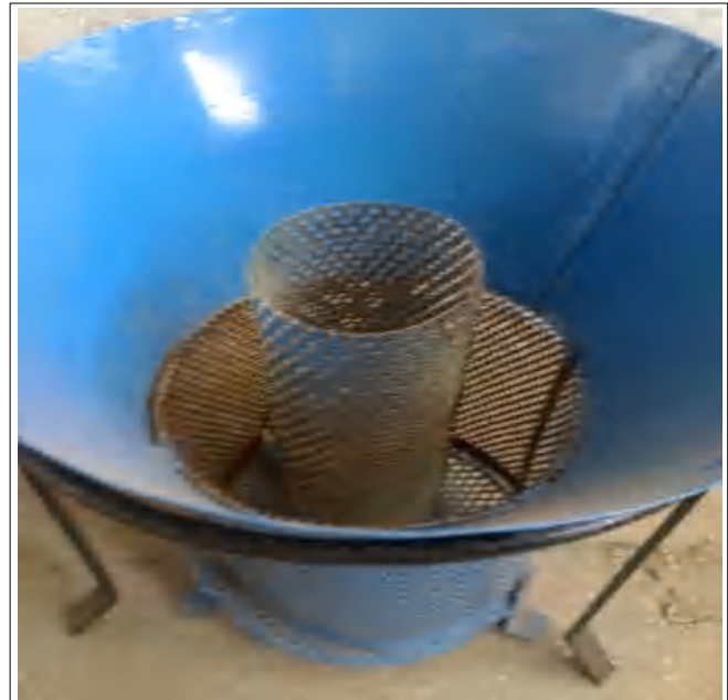
Fig. C : Husk cook stove with central port made up of stainless steel
