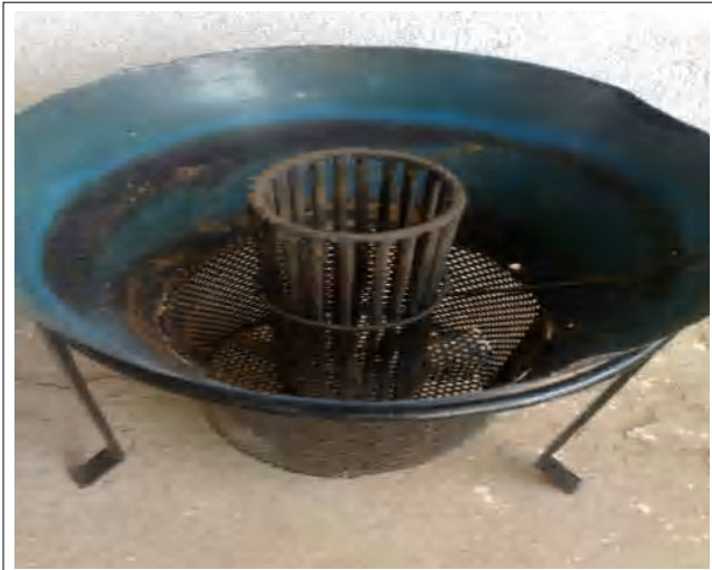
Fig. A : Husk cook stove with central port made up of MS rod
