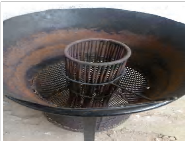
Fig. B : Husk cook stove with central port made up of GI wire
