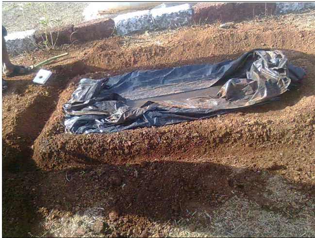
Plate A: Basin prepared in soil for W-shape solar still on soil
