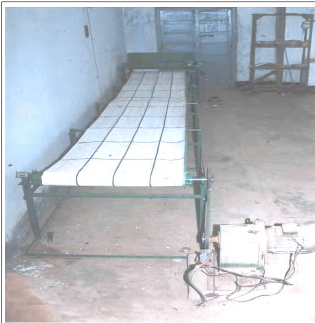
Fig. A : Test rig for metering of seeds through sticky belt
