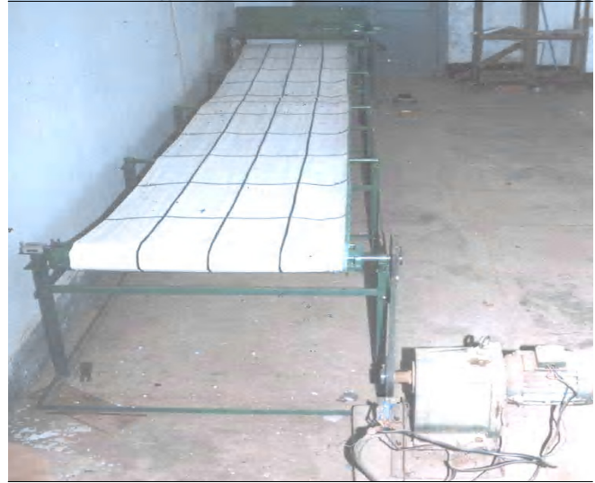
Fig. A : Test rig for metering of seeds through sticky belt
