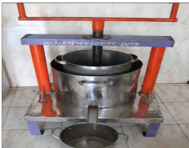
Plate B : Basket press for extraction of cashew apple juice
