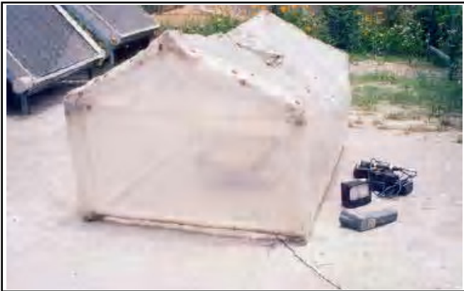
Fig. 1 : Experimental set-up for prawn drying inside greenhouse
