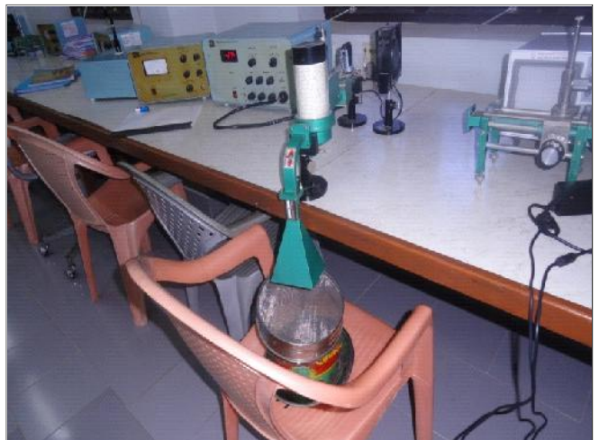
Fig. H: Radiation protection test using porous shield
