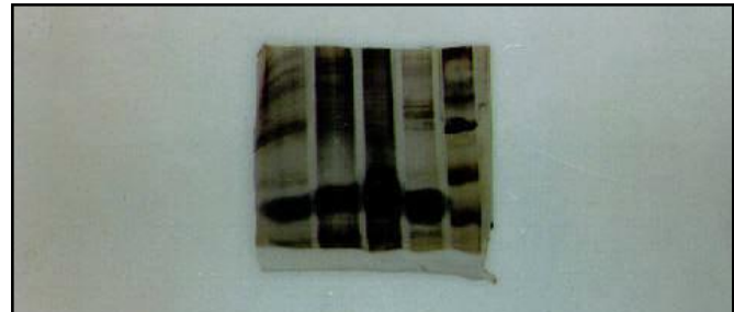
Lane 1 - crude enzyme Lane 2 - Acetone extract Lane 3 - 50% ammonium sulphate precipitation Lane 4 - 70% ammonium sulphate precipitation Lane 5 - Standard molecular weight markers E. coli galactosidase
