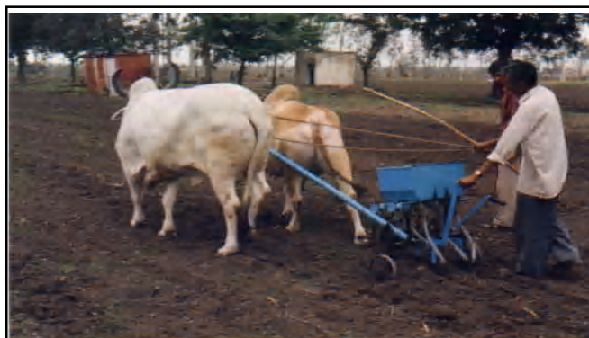
Fig. 3 : Field trial of modified rice cum green manure seeder
