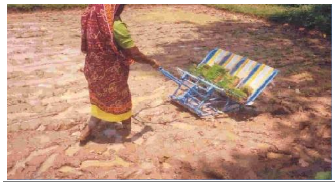
Fig. A : Operation of manually operated four row paddy transplanter
