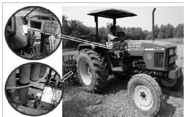
1. Oscilloscope 3. Optoelectric sensor 4. Optical sensor box
