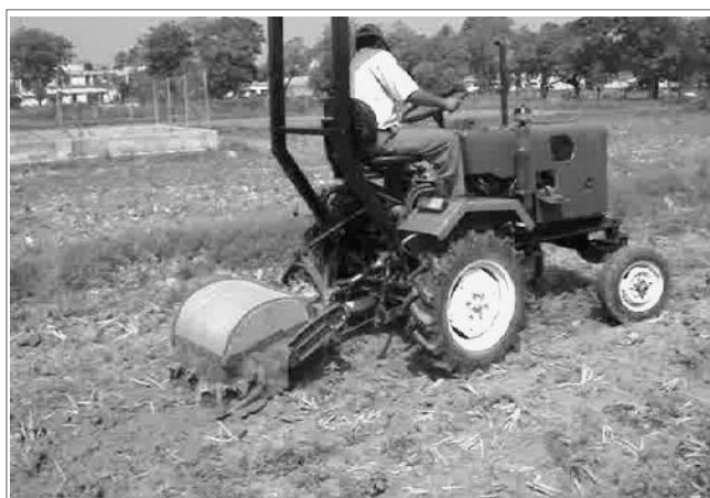
Fig. 1 : Developed rotavator with IIT mini tractor during one of the filed trail
