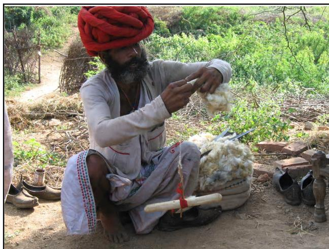
**Fig. 3 : Manual spinning technique with “Dhera”**
