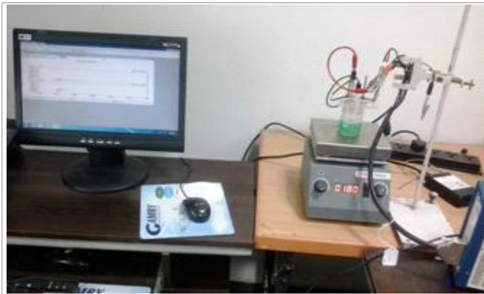
Fig. A : Systematic arrangement of electrocodeposition of Ni-TiO 2 coating
