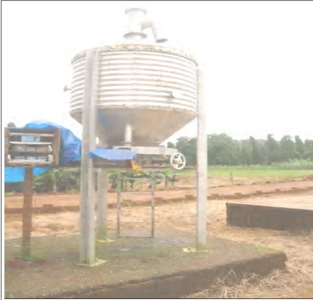
Fig. A : Galvanized Iron Corrugated structure for storage of paddy
