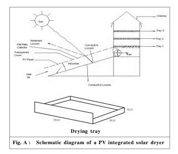
an inclination of  $30^{\circ}$  for receiving maximum solar radiation. A fan has been provided in order to extract the heated air available below the air heater and supplying that air into the drying chamber where materials to be dried are placed into the three trays.
