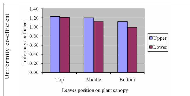
Fig. 5: Uniformity co-efficient at three position of the plant for nozzle discharge rate of 0.90 l/min and pressure 689.5 kPa for boom sprayer
