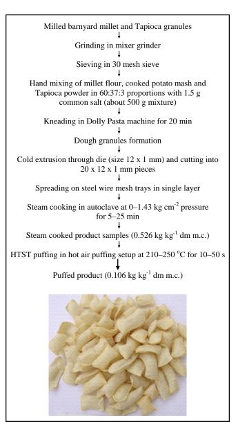
Fig. A : Process flow chart for preparation of barnyard millet puffed product
