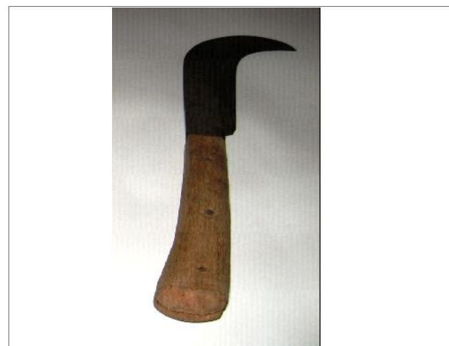
Fig. 4 : Improved pruning knife for light pruning
