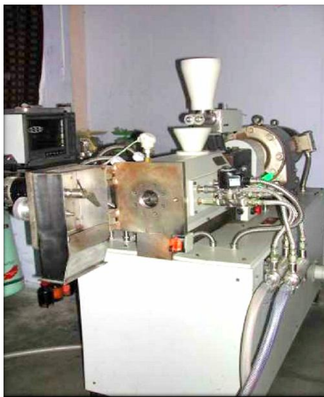
Plate 1 : Twin screw extruder BTPL model used for preparation of RTE extruded snacks during investigation
