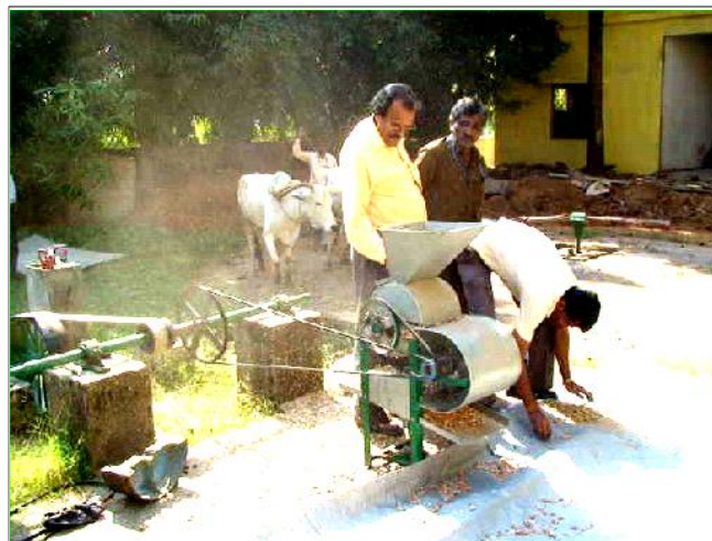
Fig. B : Operation of groundnut decorticator cum cleaner through rotary mode by using bullock power
