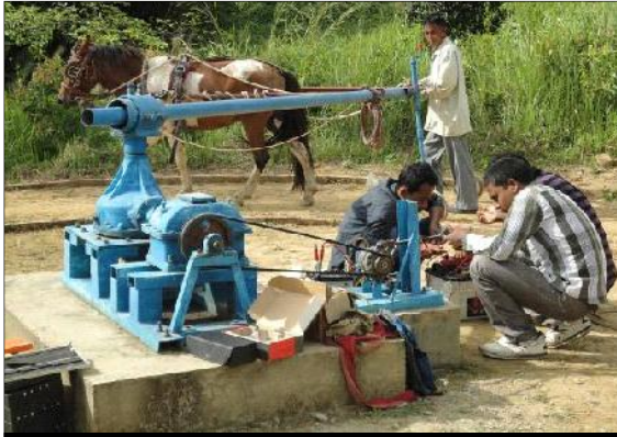
Fig. A : Rotary unit in operation at Krishi Vigyan Kendra, Andro
