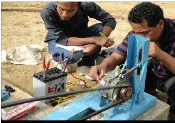
Fig. B : Measurement of current and voltage of Alternator
