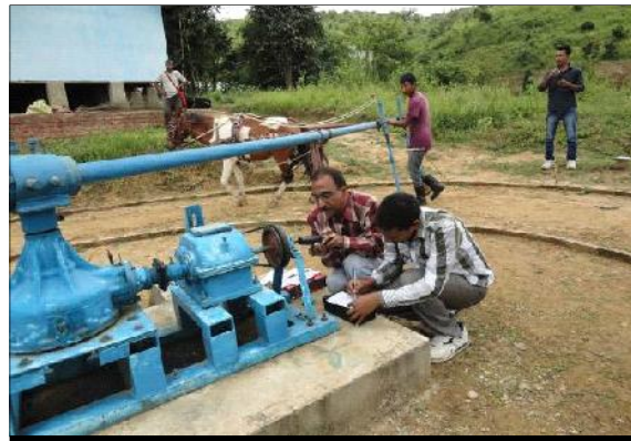
Fig. F : Speed measurement using tachometer at pulley
