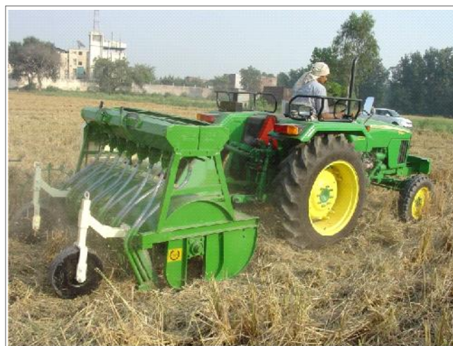
Fig. B: Sowing of farmer participatory trials with Happy seeder
