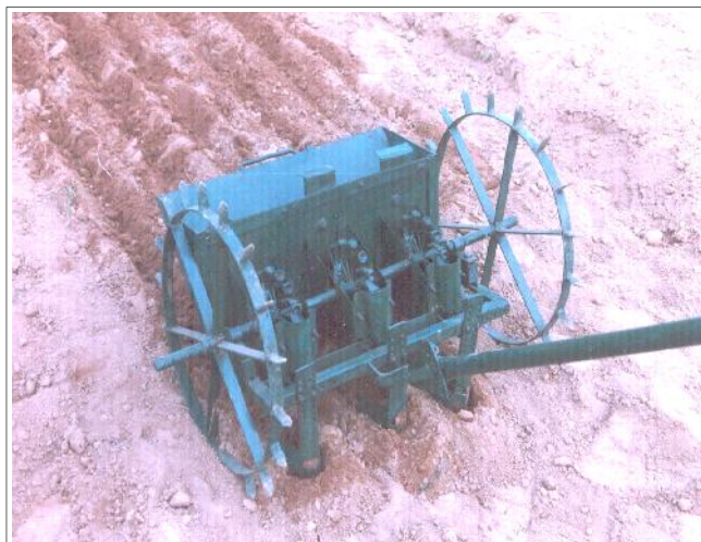
Fig. A : Field evaluation of manually operated seed drill
