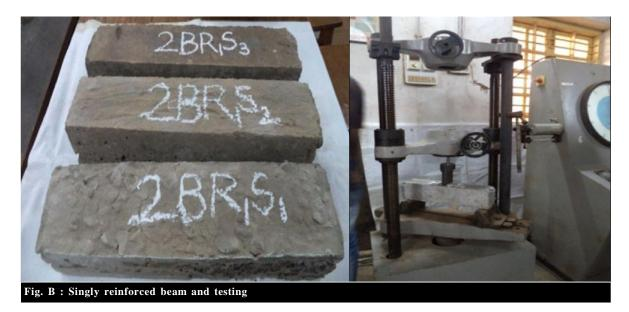
of cement. It consists of control of temperature and of the moisture movement from and into concrete. The strength of concrete gradually increases with age with proper curing. Prepared samples are kept in curing for 28 days period.
