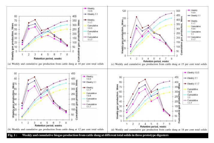
weekly gas production fluctuated marginally from first to sixth week and thereafter it decreased gradually till the retention period of eighth week in all the three prototype digesters (Fig. 1d).
