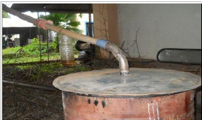
Fig. C : Oil drum kiln to produce bamboo vinegar
