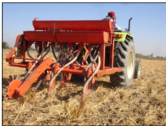
Fig. E : Sowing of wheat with spatially modified no till drill
