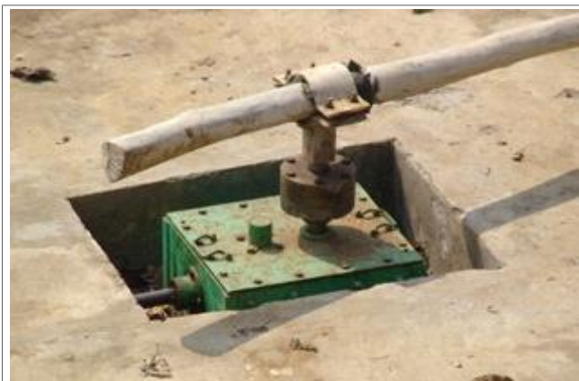
Fig. A : Gear box unit for mechanical power transmission in rotary mode
