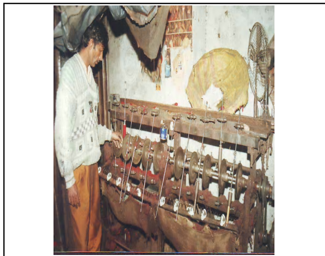
Fig. 2 : Indigenous Pirn Winding Machine
