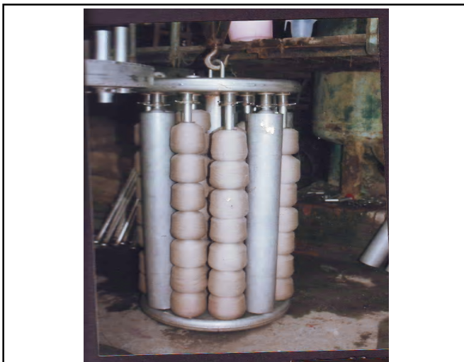
Fig. 4 : Undyed cones of yarn fitted on steel rods of carrier of Dyeing Machine
