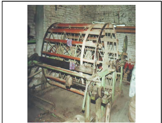
Fig. 5 : Warping Machine, its Drum and Guide Roller
