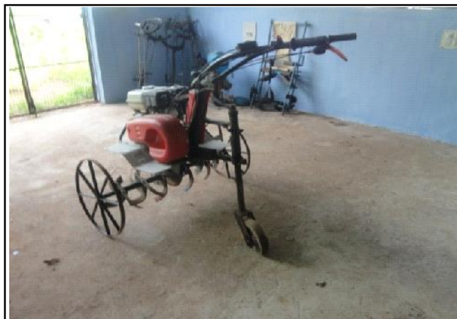
Fig. 1b : Power weeder after modification
