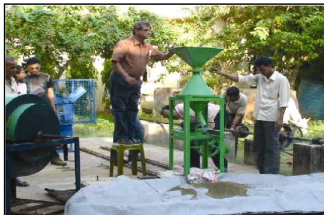
Fig. B : Photograph of operation of dhal mill through rotary mode by using bullock power
