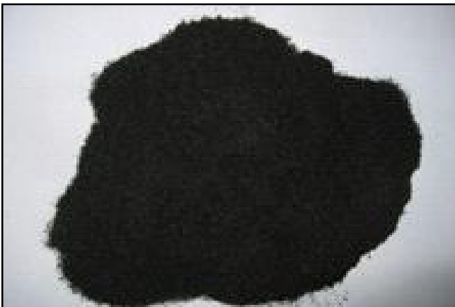
Fig. 2 : Carbonized rice husk ash abbreviated as RHA will be obtained after burning the rusk husk and it is a major source of silica
