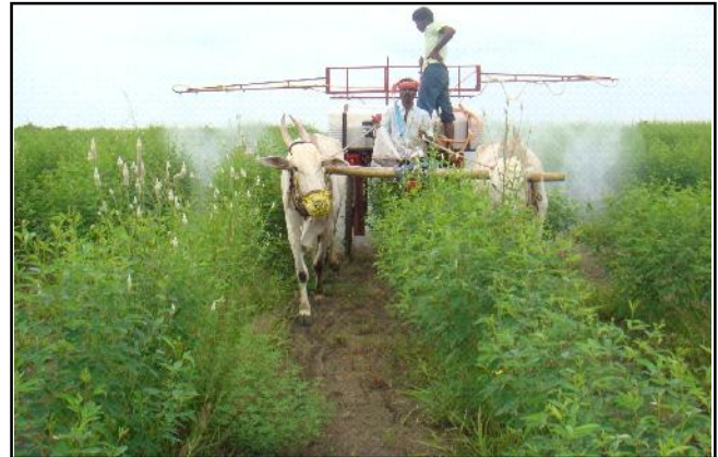
Plate 2 : Working of bullock drawn engine operated sprayer for pigeonpea crop in the farmers field
