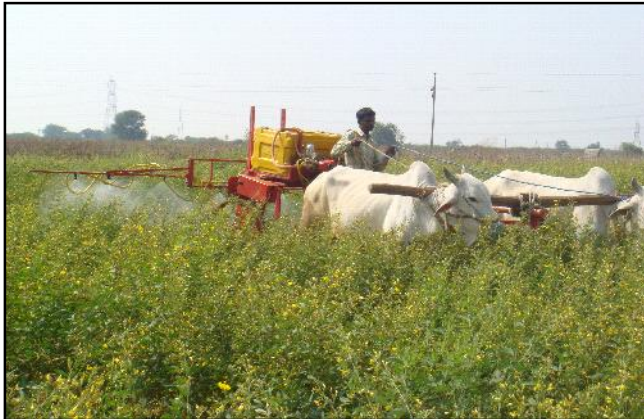
Plate 1 : A view of bullock drawn engine operated sprayer for pigeonpea crop in the research farm
