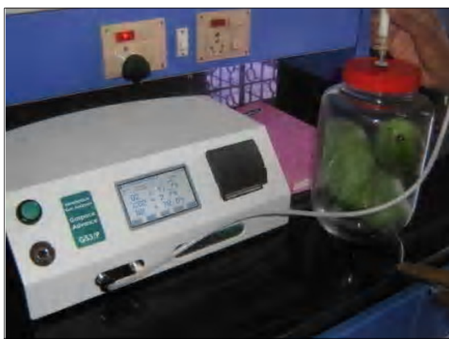
Fig. 1: A closed system for respiration rate measurement of the green mature mango
