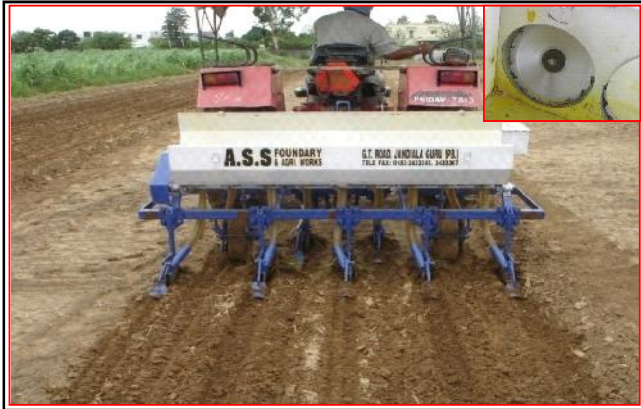
Fig. A : Direct sowing of paddy with Inclined plate planter in moist seed bed
