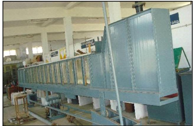
Plate A : Hydraulic flume used for experimentation
