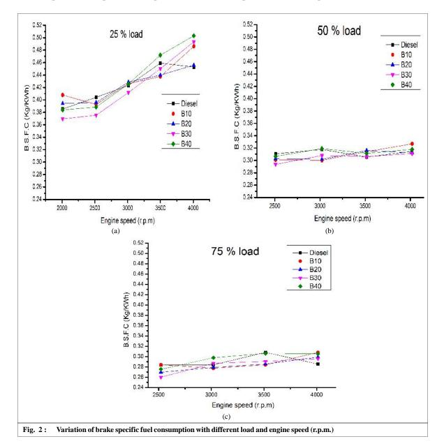
lowest value of BSFC (0.26kg/KWh) as compared to other biodiesel blends and diesel (0.28 kg/kWh)
