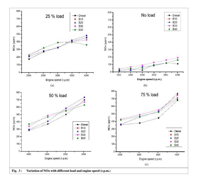
NOx for biodiesel than diesel stated higher ignition delay of biodiesel as a reason. The maximum increase of 18.30 per cent is observed for B30 at 75 per cent load @2500 rpm and maximum decrease of 20.8 per cent is found for B40 at 25 per cent load @ 4000 rpm as compared to diesel fuel.
