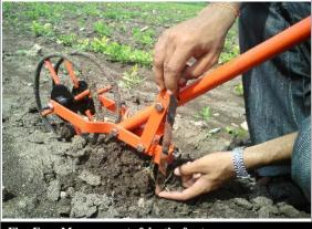
Fig. E: Measurement of depth of cut
