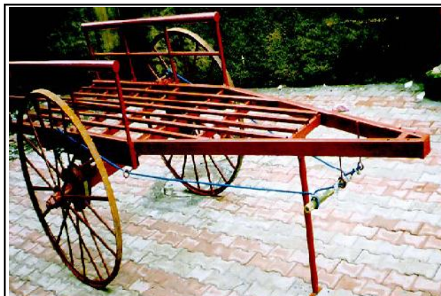
Fig. A : two wheel steel cart (2.0 tones capacity) without rubber liner on its wheel
