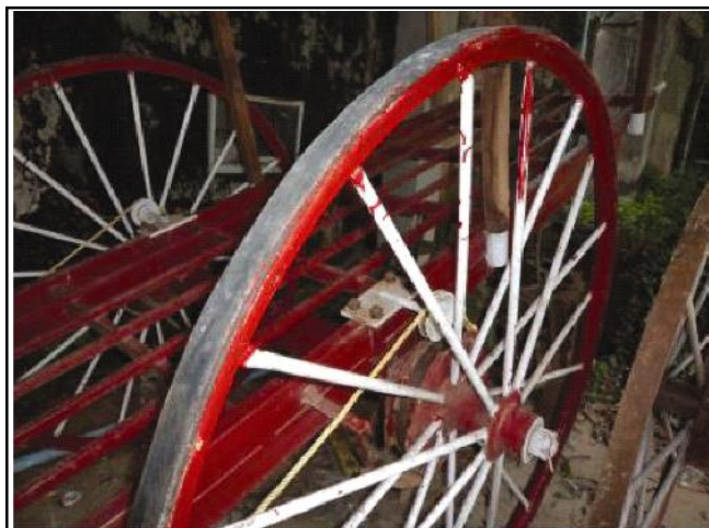
Fig. B : Two wheel steel cart (2.0 tones capacity) with rubber liner on its wheel
