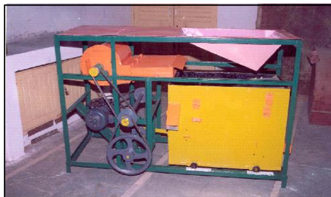
Fig. 1 : Developed cumin cleaner cum grader
