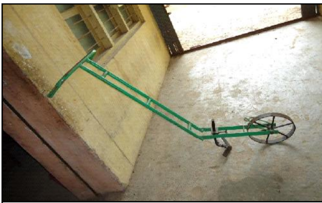
Fig. B : Schematic diagram of wheel hoe
