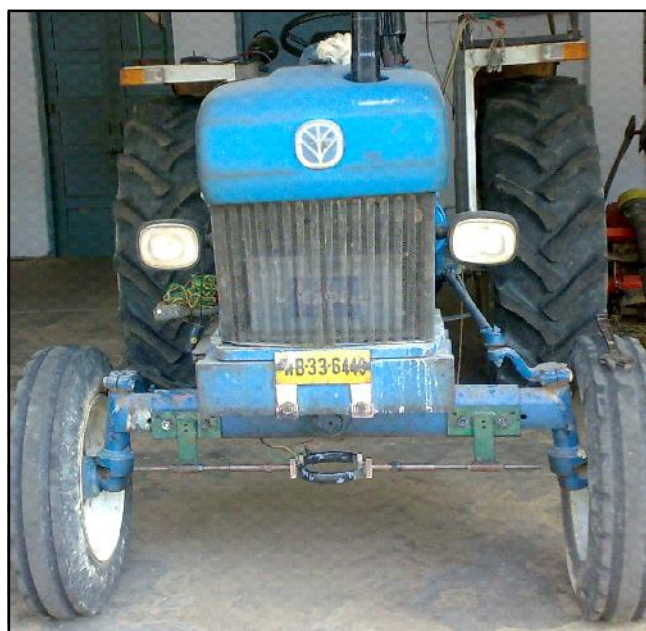
Fig. A : Attachment of ring transducer to the front axle of tractor
