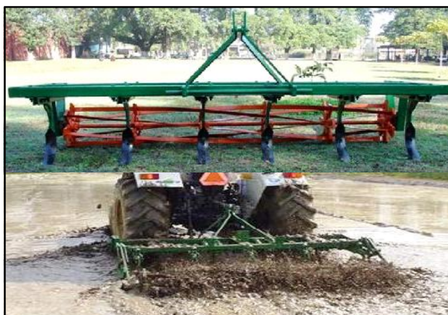
Fig. A : A stationary and working view of pulverizing roller
