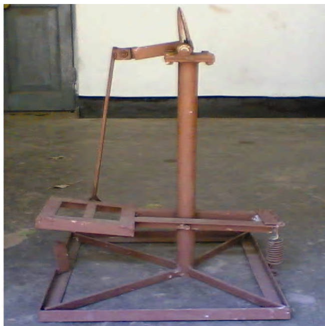
Fig. 2 : Photograph of pedal operated coconut dehusker
