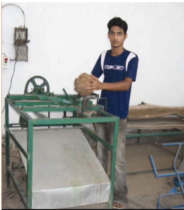
Fig. 4 : Working of power operated coconut dehusker
