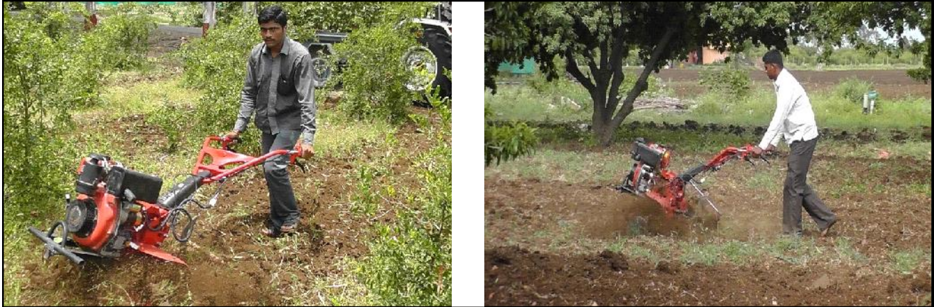
Fig. B : Operation of self propelled rotary weeder in pomegranate and sapota crop field
