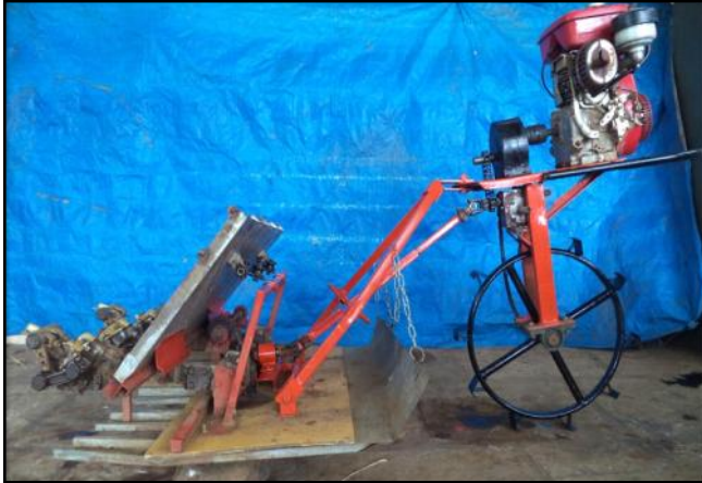
Fig. B : Developed four row self propelled paddy transplanter
