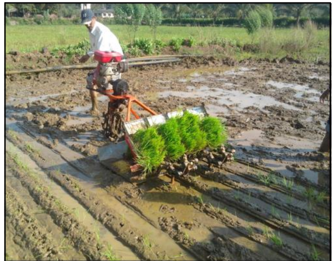
Fig. C : Field testing of newly developed four row self propelled paddy transplanter
