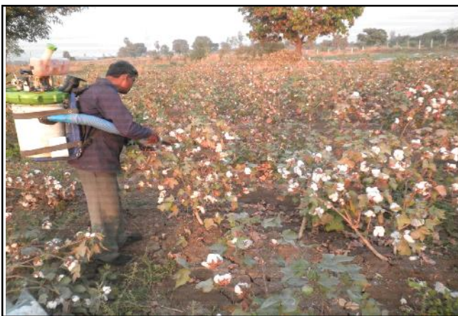
Fig. C : Field testing of cotton picker
