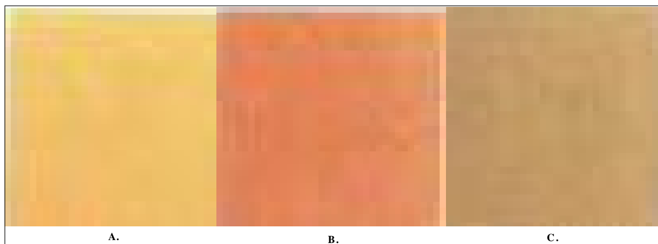
Fig. 3 : Shades obtained with turmeric treatment with (A) no mordant (B) Potassium Aluminum sulphate and (C) Copper sulphate
